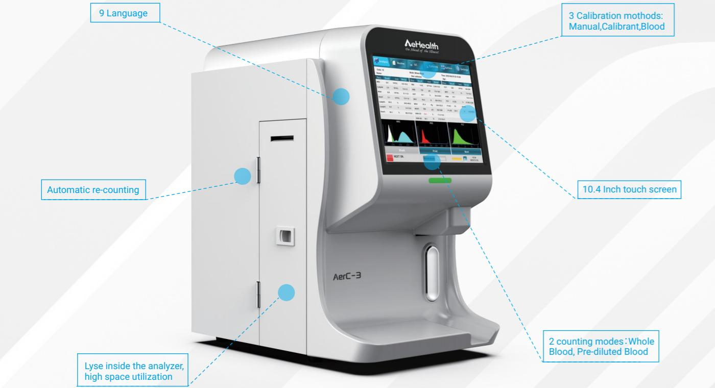
AerC-3 Auto Hematology Analyzer is a clinical test instrument with rich functions and easy operation. It can provide 21 parameters and 3 histograms. Double channel counting. During the sample analysis process, automatic blockage removal and automatic re-counting ensure accurate and stable test results. Widely used in hospital laboratories, clinical departments and research centers.
